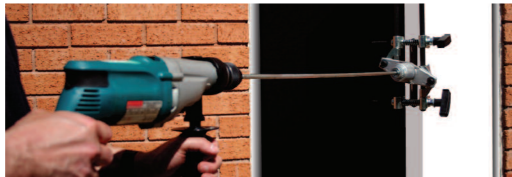
Long Drill Adapter installed on housing
